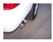
8. INSTALL YOUR BLACK CERAMIC COATED TIPS. PROCEED TO THE NEXT SHEET ON HOW TO INSTALL YOUR DEEGAN 38 BADGES. AFTER YOU HAVE CHECKED FOR CLEARANCES GO BACK AND TIGHTEN ALL NUTS, BOLTS AND CLAMPS.
