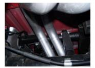
6. Slide the driver side over axle tailpipe #D into the muffler 1.5-2". Use clamp #G to secure tailpipe to muffler. Do not tighten. Insert welded hanger into rubber grommet.
