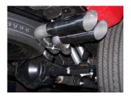
7. Attach tailpipes together with bolt kit #H. Driver side tab should be on the bottom.
