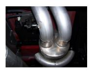
4. Slide muffler #B over headpipe 1.5-2" with the louvers facing towards the converter. Use a jack stand to support the muffler. Use clamp #F to secure the muffler to the headpipe. Do not tighten. Muffler inlet is looking into the louvers.
