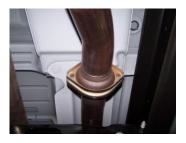
2. To remove your stock exhaust, unbolt the 2-bolt flange located in front of the muffler. Disengage the welded hangers from the rubber grommets. Use WD-40 to aid in this process. Do not remove or damage the rubber grommets as you will reuse them to mount your new system. Now, cut off tailpipe and remove exhaust. Do not throw away stock hardware.
