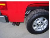
8. INSTALL YOUR BLACK CERAMIC COATED TIPS. PROCEED TO THE NEXT SHEET ON HOW TO INSTALL YOUR DEEGAN 38 BADGES. AFTER YOU HAVE CHECKED FOR CLEARANCES GO BACK AND TIGHTEN ALL NUTS, BOLTS AND CLAMPS..
