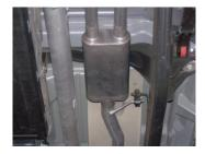
4. Install muffler #B with inlet towards Y-pipe. Use jack stands to support the muffler. Use clamp #F to secure the muffler to headpipe. Do not tighten.
