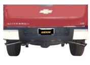
Install stainless steel tips. Clamp down. When you have everything in place, firmly tighten all bolts and clamps down securely. Use stainless steel cleaner and a Scotch Brite pad weekly to prevent tip from discoloration. Inspect all fasteners after 25-50 miles of operation and re-tighten as necessary.
