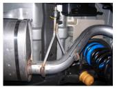
**2.** To remove the stock exhaust, remove it from the clamp in front of the muffler. Do not destroy you will re-use clamp. Disengage the welded hangers using WD-40 from the OEM rubber grommets. Do not damage or remove the rubber grommets as you will reuse them to mount your new system. Now, cut off tailpipe before and after rear axle for
