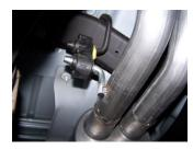
**6.** Install Driver side tailpipe #C into muffler outlet 11/2-2". Insert welded hanger into rubber grommet. Use clamp #F to attach tailpipe to muffler. DO NOT TIGHTEN.
