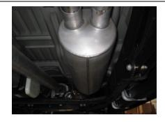
3. Install muffler #B onto headpipe 1.5" to 2" muffler should be level use clamp #E to secure together do not tighten.
