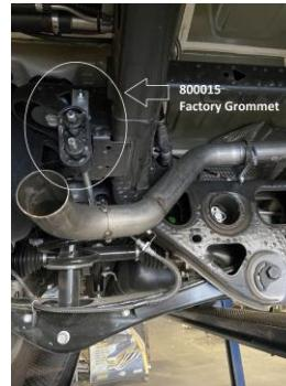
Install metal hangers #K using Bolt Kit #J. We will Re-use the middle support hanger grommet from the stock exhaust for this bracket.
