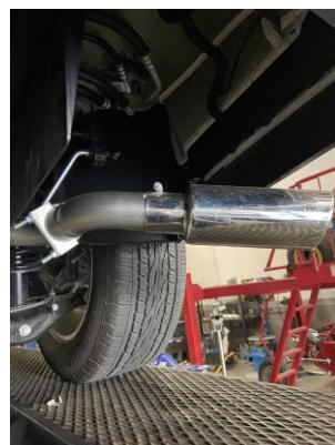
Install the Over Axle (B) #D onto the PS output of the First Over Axle Pipe then install Over Axle (C). Use clamps #G to secure pipe. Do not tighten. Next, Install the Exit Pipes #E with the tips pre-installed to set height, then tighten using clamps #G.
