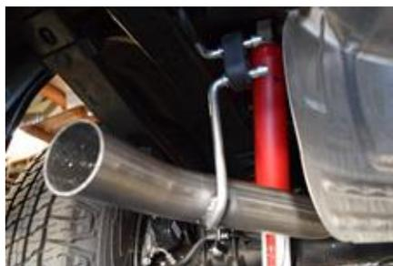
5. Before install of item E, install Driver side hanger bracket as shown in picture. Install supplied 2-1/2" band clamp onto the inlet side of the driver side over-axle pipe A and install onto outlet of muffler. Install hanger into factory rubber grommet hanger. Next install another 2-1/2" band clamp onto the inlet side of driver side over-axle pipe B (Item E) and install onto outlet of Item D. Tighten both clamps with allowance for adjustment.
