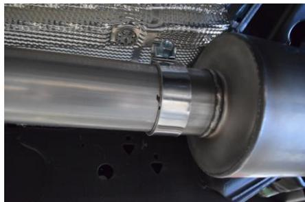
3. Install supplied 3" clamp (Item H) onto inlet end of new muffler (Item B) and slip onto end of the head pipe with 2-1/4" inserted into muffler. Tighten with allowance for adjustment.
