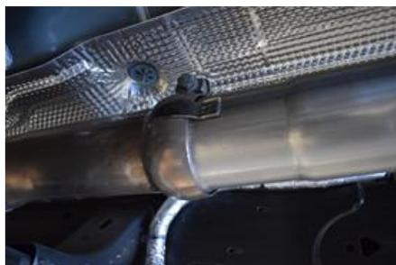
2. Remove clamp from factory head pipe using a small flathead screwdriver to bend up the retaining clip and then install onto new head pipe (Item A). Next, install head pipe and tighten with allowance for adjustment.
