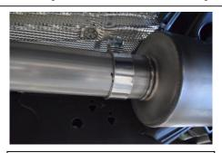
3. Install supplied 3" clamp(Item H) onto inlet end of new muffler(Item B) and slip onto end of the head pipe with 2-1/4" inserted into muffler. Tighten with allowance for adjustment.
