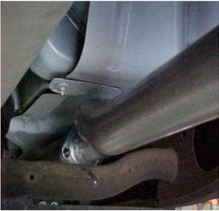
Install head pipe # A onto you're existing stock flange re-using the factory hardware. Use a jack stand to support the converter. Do not tighten. Insert welded hanger into rubber grommet.
