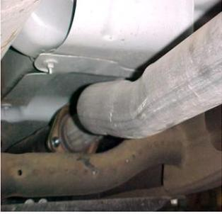
Lay out the exhaust on the floor so it looks like the drawing and compare parts with manual. To remove the stock exhaust un-bolt it from the flange located in front of the muffler. **You will re-use your stock hardware.** Leave all rubber grommets in place. Use WD-40 to aid in removal of exhaust and the hangers. Cut your stock tailpipe off just behind the muffler.
