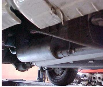
Install the driver side over axle tailpipe # D into the muffler. Use clamp # F to secure tailpipe to muffler. Do not tighten. Insert hanger into rubber grommet.
