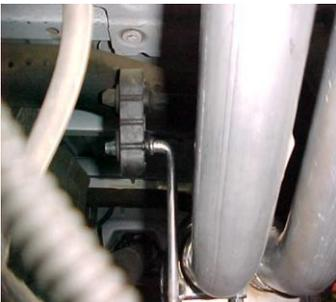
Install muffler onto head pipe 1-1/2" to 2" with the louvers facing towards the converter. Use a jack stand to support the muffler. Use clamp # F to secure the muffler to the head pipe. Do not tighten.
