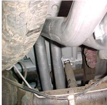
Install passenger side over axle tailpipe # C into muffler and attach using clamp # G. Insert welded hanger into rubber grommet. Use bolt kit # H to attach the tailpipes together. Do not tighten. YOU MAY NEED TO LOOSEN YOUR SPARE TIRE & PUSH TOWRDS DRIVER SIDE & RE-TIGHTEN
