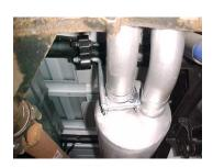
Install muffler #C onto head pipe #B 1-1/2" to 2" with the louvers facing towards the converter. Use a jack stand to support the muffler. Use clamp #G to secure the muffler to the head pipe. Do not tighten. Install rear muffler hanger #I onto driverside muffler outlet. Insert hanger into rubber grommet. Do not tighten.
