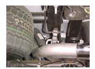
Install the passenger side over axle tailpipe #D into the muffler 1 ½" to 2". Use clamp #H to secure tailpipe to muffler. Do not tighten. Insert welded hanger into rubber grommet
