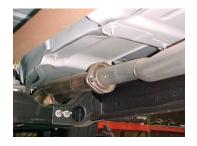
Lay out the exhaust on the floor so it looks like the drawing and compare parts with manual. To remove the stock exhaust un-bolt it from the 2-bolt flange located behind your factory Y-pipe. You will re-use your factory hardware. Leave all rubber grommets in place. Use WD-40 to aid in removal of exhaust and the hangers. Now cut off your stock tailpipe just behind the muffler.
