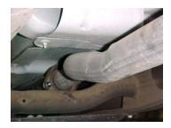
Lay out the exhaust on the floor so it looks like the drawing and compare parts with manual. To remove the stock exhaust un-bolt it from the flange located in front of the muffler. You will re-use your stock hardware. Leave all rubber grommets in place. Use WD-40 to aid in removal of exhaust and the hangers. Cut your stock tailpipe off just
