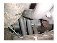
Install passenger side over axle tailpipe # C into muffler and attach using clamp # H. Use bolt kit # I to attach the tailpipes together. Do not tighten. YOU MAY NEED TO LOOSEN YOUR SPARE TIRE & PUSH TOWRDS DRIVER SIDE & RE-TIGHTEN
