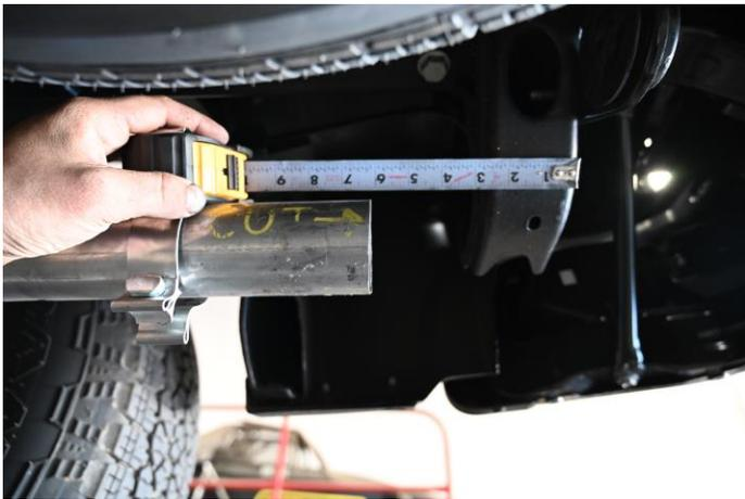
**3)** THIRD, CUT PASSENGER SIDE OUTLET PIPE 6" FROM THE REAR LEAF SPRING MOUNTING BUCKET
