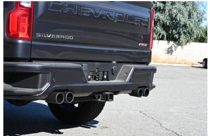
**4)** FINALLY, ADJUST TIPS TO DESIRED LOOK AND DEPTH THEN TIGHTEN. **NOTE: THESE TIPS HAVE AN EXCEPTIONAL AMOUNT OF DEPTH ADJUSTMENT**
