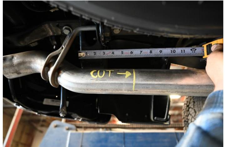
**2)** SECOND, CUT DRIVER SIDE OUTLET PIPE 6" FROM THE REAR LEAF SPRING BUCKET.
