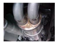
Install muffler #C onto head pipes 1-1/2" to 2" with the louvers facing towards the converter. The inlets and outlets of the muffler will be on the bottom. Use a jack stand to support the muffler. Use clamp #H to secure the muffler to the head pipe. Do not tighten. Muffler inlet is looking into the louvers.
