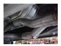
Install head pipe #A onto passenger side stock pipe and insert hanger into rubber grommet. Next install driver side head pipe #B onto drivers side factory pipe. Use clamp #H to secure pipes together. Do not tighten.
