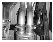
INSTALL PASSENGER TAILPIPE #D IN THE REAR OF THE MUFFLER. USE CLAMP # G TO ATTACH PASSENGER TAILPIPE TO. DO NOT TIGHTEN.
