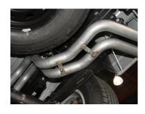
INSTALL PASSENGER SIDE TAILPIPE #D INTO MUFFLER AND ATTACH USING CLAMP #F. INSERT WELDED HANGER INTO RUBBER GROMMET. DO NOT TIGHTEN. USE BOLT KIT #I TO ATTACH THE TAILPIPES TOGETHER. DO NOT TIGHTEN. DRIVERSIDE TAILPIPE TABS WILL BE ON THE BOTTOM.
