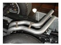
INSTALL DRIVERSIDE TAILPIPE #C INTO MUFFLER. USE CLAMP #F TO SECURE TAILPIPE TO MUFFLER.
