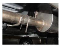
TO REMOVE THE STOCK EXHAUST UNCLAMP THE STOCK EXHAUST JUST IN FRONT OF THE MUFFLER. YOU MAY NEED TO HEAT IT UP FOR EASIER REMOVAL. LEAVE ALL RUBBER GROMMETS IN PLACE. USE WD-40 FOR REMOVAL OF HANGERS.
