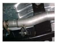
INSTALL HEADPIPE #A ONTO YOUR EXISTING STOCK FRONT PIPE AND SECURE WITH CLAMP #F. USE A JACKSTAND TO SUPPORT THE CONVERTER. INSERT WELDED HANGER INTO RUBBER GROMMET.
