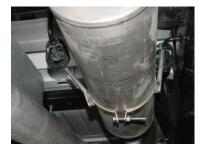
INSTALL MUFFLER #B ONTO HEADPIPE #A 1-1/2" TO 2". USE CLAMP #G TO SECURE THE MUFFLER TO THE HEADPIPE. DO NOT TIGHTEN. SLIDE BAND CLAMP #H ONTO THE MUFFLER AND INSERT THE WELDED HANGERS INTO THE RUBBER GROMMETS AND ATTACH WITH BOLT KIT # J.
