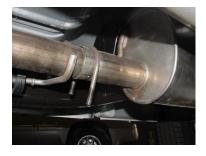
TO REMOVE THE STOCK EXHAUST UNCLAMP THE STOCK EXHAUST JUST IN FRONT OF THE MUFFLER. YOU MAY NEED TO HEAT IT UP FOR EASIER REMOVAL. LEAVE ALL RUBBER GROMMETS IN PLACE. USE WD-40 FOR REMOVAL OF HANGERS.
