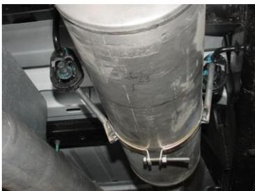
INSTALL MUFFLER #B ONTO HEADPIPE 1-1/2" TO 2". USE CLAMP #G TO SECURE THE MUFFLER TO THE HEADPIPE. DO NOT TIGHTEN. SLIDE BAND CLAMP #H ONTO THE MUFFLER AND INSERT THE WELDED HANGERS INTO THE RUBBER GROMMETS AND ATTACH WITH BOLT KIT #J.
