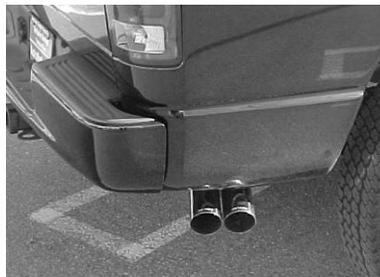
INSTALL THE STAINLESS TIPS. NOW GO BACK AND TIGHTEN ALL CLAMPS, NUTS AND BOLTS STARTING FROM THE FRONT AND WORKING BACK. TO CLEAN TIPS USE A SCOTCH BRITE PAD AND ANY STAINLESS CLEANER.
