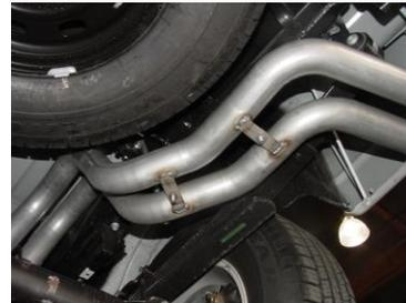
INSTALL PASSENGER SIDE TAILPIPE #D INTO MUFFLER AND ATTACH USING CLAMP #F. INSERT WELDED HANGER INTO RUBBER GROMMET. DO NOT TIGHTEN. USE BOLT KIT #I TO ATTACH THE TAILPIPES TOGETHER. DO NOT TIGHTEN. PASSANGER SIDE TABS ON THE TAILPIPE WILL BE ON TOP OF THE DRIVERSIDE TABS.
