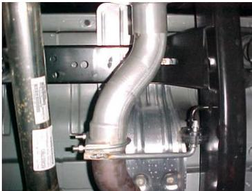
INSTALL HEADPIPE #A ONTO YOUR EXISTING STOCK FRONT PIPE AND SECURE WITH CLAMP #K. USE A JACKSTAND TO SUPPORT THE CONVERTER. INSERT WELDED HANGER INTO RUBBER GROMMET.
