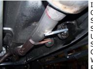
INSTALL HEADPIPE #A ONTO YOUR EXISTING STOCK FRONT PIPE AND SECURE WITH CLAMP #K. USE A JACKSTAND TO SUPPORT THE CONVERTER. INSERT WELDED HANGER INTO RUBBER GROMMET. DO NOT TIGHTEN.
