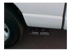
INSTALL YOUR STAINLESS TIPS. THERE IS A LEFT AND A RIGHT TIP. TIGHTEN ALL CLAMPS AFTER YOU MAKE SURE YOUR TAILPIPES ARE LEVEL.
