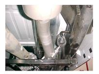
INSTALL HEADPIPE #A ONTO YOUR EXISTING STOCK FRONT PIPE AND SECURE WITH CLAMP #G. USE A JACKSTAND TO SUPPORT THE CONVERTER. INSERT WELDED HANGER INTO RUBBER GROMMET.
