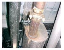
YOU MAY NEED TO HEAT IT UP FOR EASIER REMOVAL. LEAVE ALL RUBBER GROMMETS IN PLACE. USE WD-40 FOR REMOVAL OF HANGERS. FOR EASIER REMOVAL, REMOVE THE TWO CROSSMEMBER BARS FIRST.
