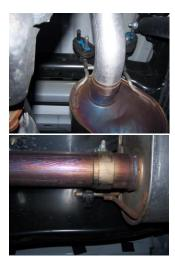
**1.** To remove the stock exhaust un-clamp the tailpipe just after the stock muffler. Then un-clamp the stock muffler. Leave all rubber grommets in place. Use WD-40 to aid in removal of exhaust.
