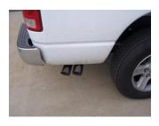
6. INSTALL YOUR BLACK CERAMIC COATED TIPS. PROCEED TO THE NEXT SHEET ON HOW TO INSTALL YOUR DEEGAN 38 BADGES. AFTER YOU HAVE CHECKED FOR CLEARANCES GO BACK AND TIGHTEN ALL NUTS, BOLTS AND CLAMPS.
