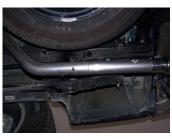
6. Install the passenger side over axle tailpipe #C into the muffler 1.5-2". Use clamp #H to secure. Do not tighten. Insert welded hanger into rubber grommet.
