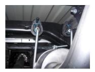
5. Slide band clamp #J onto muffler #B and attach with bolt kit #M. Do not tighten. Insert hangers into rubber grommets.
