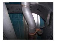
3. Install headpipe #A onto your existing stock headpipe and attach with clamp #I. Do not tighten. Use a jack stand to support the converter.
