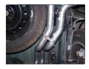
**7.** Attach tailpipes together with bolt kits #I. DO NOT TIGHTEN. Driver side tabs will be on bottom.
