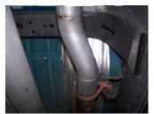
**2.** Install head pipe #A onto your existing stock front pipe and attach with clamp #G. Use a jack stand to support the converter.
