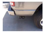
**8.** Install stainless steel tips #E. Clamp down. When you have everything in place, firmly tighten all bolts and clamps down securely. Use stainless steel cleaner and a Scotch Brite pad weekly to prevent tip from discoloration.
