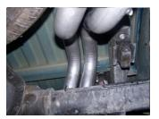
**6.** Install the driver side overaxle tailpipe #C into the muffler 1½"-2". Use clamp #F to secure tailpipe to muffler. DO NOT TIGHTEN.
