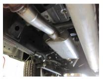
3. Install Head Pipe #A onto your factory pipe. Insert welded hanger into factory rubber grommet. Use Clamp # F to secure. Do not tighten.
