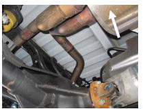
2. To remove the stock exhaust, remove it from the clamp in front of the muffler. Disengage the welded hangers using WD-40 from the OEM rubber grommets. Do not damage or remove the rubber grommets as vou will reuse them to mount your new system.
