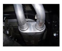
4. Install muffler #B onto head pipe #A 11/2"-2". Use a jack stand to support the muffler. Use clamp #F to secure the muffler to the headpipe. DO NOT TIGHTEN.
