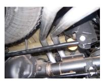
**7.** Install Driver side tailpipe #D into the muffler 1½-2". Use clamp #G to secure tailpipe to muffler. DO NOT TIGHTEN. Insert welded hangers into rubber grommets. Use bolt kit # H to attach both tailpipes.
