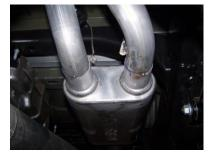
**4.** Install muffler #B onto head pipe #A  $1\frac{1}{2}$ "-2". Use a jack stand to support the muffler. Use clamp #F to secure the muffler to the headpipe. DO NOT TIGHTEN.
