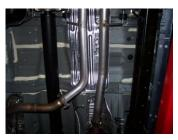
3. Install passenger side headpipe #A using your stock bolts. Do not tighten. Next. install driver side headpipe #B (2009+ models use #K) using stock bolts. Do not tighten. Install metal hangers into rubber grommets.
