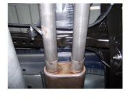
5. Install extension pipe #D into muffler. Use clamp #I to secure. Do not tighten. Next install driver side extension pipe #E into muffler using clamp #I to secure. Do not tighten. Insert welded hanger into rubber grommet.
