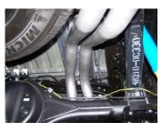
7. Install driver side over axle tailpipe #G onto extension pipe. Use clamp #I to secure the pipe. Do not tighten.
