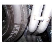
8. Use bolt kit #J to secure tabs. Make sure driver side tab is on the bottom. (You may need to loosen up the spare tire and move it over for better clearance.)
