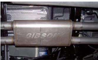
5. Install extension pipe #D into muffler. Use clamp #I to secure. Do not tighten. Next install driver side extension pipe #E into muffler using clamp #I to secure. Do not tighten. Insert welded hanger into rubber grommet.
