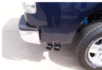
9. Install stainless steel tips. Clamp down. When you have everything in place, firmly tighten all bolts and clamps down securely. Use stainless steel cleaner and a Scotch Brite pad weekly to prevent tip from discoloration. Inspect all fasteners after 25-50 miles of operation and re-tighten as necessary.
