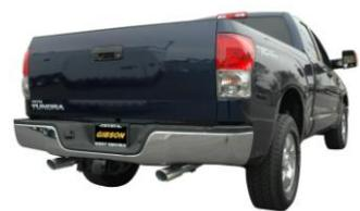
10. Install stainless steel tips. Clamp down. When you have everything in place, firmly tighten all bolts and clamps down securely. Use stainless steel cleaner and a Scotch Brite pad weekly to prevent tip from discoloration. Inspect all fasteners after 25-50 miles of operation and re-tighten as necessary.
