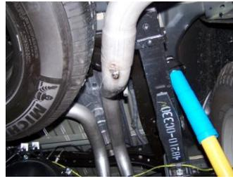
6. Install the passenger side overaxle tailpipe #F to the extension pipe. Use clamp #J to secure. Do not tighten. Insert welded hanger into rubber grommet.
