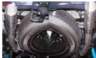
9. Next, install the exit pipes #H. Use clamps #J to secure the tailpipes.
