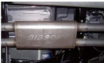
5. Install extension pipe #D into muffler. Use clamp #J to secure. Do not tighten. Next install driver side extension pipe #E into muffler using clamp #J to secure. Do not tighten. Insert welded hanger into rubber grommet.
