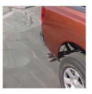
INSTALL YOUR BLACK CERAMIC COATED TIPS. PROCEED TO THE NEXT SHEET ON HOW TO INSTALL YOUR DEEGAN 38 BADGES. AFTER YOU HAVE CHECKED FOR CLEARANCES GO BACK AND TIGHTEN ALL NUTS, BOLTS AND CLAMPS..
