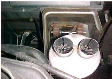
**SLIP MUFFLER # B THROUGH BAND CLAMP THEN ONTO THE HEADPIPE 1 1/2" TO 2". THE OUTLETS WILL BE ON THE TOP. USE CLAMP # F TO SECURE MUFFLER TO HEADPIPE. DO NOT TIGHTEN.**
