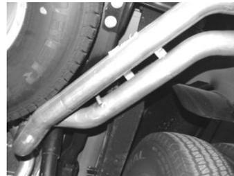
**NEXT INSTALL PASSENGER OVER AXLE PIPE # C INTO MUFFLER 1 1/2 TO 2" IT WILL ROUTE UNDERNEATH PASSENGER SIDE TAILPIPE, AND ATTACH TO MUFFLER WITH CLAMP # G. USE BOLT KIT # I TO SECURE PIPES TOGETHER. WELDED TABS ON PASSENGER TAILPIPE WILL BE ON TOP OF OTHER PIPE TABS.**
