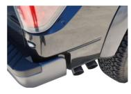
INSTALL YOUR BLACK CERAMIC COATED TIPS. PROCEED TO THE NEXT SHEET ON HOW TO INSTALL YOUR DEEGAN 38 BADGES. AFTER YOU HAVE CHECKED FOR CLEARANCES GO BACK AND TIGHTEN ALL NUTS. BOLTS AND CLAMPS.
