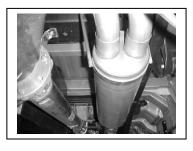
SLIP MUFFLER #B ONTO THE HEADPIPE 1 ½" TO 2". THE OUTLETS WILL BE LEVEL. USE CLAMP #G TO SECURE MUFFLER TO HEADPIPE. DO NOT TIGHTEN.
