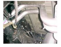
INSTALL PASS. SIDE TAILPIPE # C INTO MUFFLER 1 ½" TO 2". INSERT HANGER INTO RUBBER GROMMET, USE CLAMP # G TO SECURE PIPE TO MUFFLER. DO NOT TIGHTEN. YOU MAY NEED TO LOOSEN AND PUSH OVER TOWARDS THE DRIVERS SIDE AND RE-TIGHTEN.
