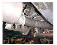
INSTALL FRONT MUFFLER HANGER # F ONTO MUFFLER INLLET, INSERT HANGER INTO RUBBER GROMMET, DO NOT TIGHTEN. USE BOLT KIT # I TO SECURE.
