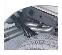
INSTALL DRIVERS SIDE TAILPIPE # D INTO MUFFLER 1  $\frac{1}{2}$ " TO 2". INSERT HANGER INTO RUBBER GROMMET, USE CLAMP # G TO SECURE PIPE TO MUFFLER. DO NOT TIGHTEN. THE TAB ON THIS PIPE SHOULD GO ON TOP OF PASSENGER SIDE PIPE USE BOLT KIT # J TO SECURE TOGETHER.
