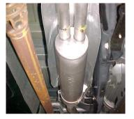
INSTALL MUFFLER # B ONTO HEADPIPE 1 <sup>1</sup>/<sub>2</sub>" TO 2". USE A JACK STAND TO HOLD UP THE MUFFLER. OUTLETS SHOULD BE ON THE TOP.
