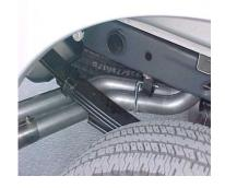
INSTALL DRIVERS SIDE TAILPIPE # D INTO MUFFLER 1 ½" TO 2". INSERT HANGER INTO RUBBER GROMMET, USE CLAMP # G TO SECURE PIPE TO MUFFLER. DO NOT TIGHTEN. THE TAB ON THIS PIPE SHOULD GO ON TOP OF PASSENGER SIDE PIPE USE BOLT KIT # J TO SECURE TOGETHER.
