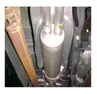
INSTALL MUFFLER # B ONTO HEADPIPE 1 ½" TO 2". USE CLAMP # F TO SECURE MUFFLER TO HEADPIPE. DO NOT TIGHTEN. USE A JACK STAND TO HOLD UP THE MUFFLER. OUTLETS SHOULD BE LEVEL.
