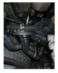
INSTALL DRIVERS SIDE TAILPIPE # D INTO MUFFLER 1 ½" TO 2". INSERT HANGERS INTO RUBBER GROMMETS, USE CLAMP # G TO SECURE PIPE TO MUFFLER. DO NOT TIGHTEN. THE TAB ON THIS PIPE SHOULD GO ON BOTTOM OF PASSENGER SIDE PIPE USE BOLT KIT # H TO SECURE TOGETHER.
