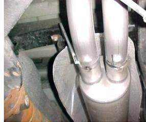
INSTALL DRIVERS SIDE TAILPIPE # D INTO MUFFLER 1 1/2" TO 2". INSERT HANGERS INTO RUBBER GROMMETS, USE CLAMP # G TO SECURE PIPE TO MUFFLER. DO NOT TIGHTEN. THE TAB ON THIS PIPE SHOULD GO ON BOTTOM OF PASSENGER SIDE PIPE USE BOLT KIT # H TO SECURE TOGETHER.
