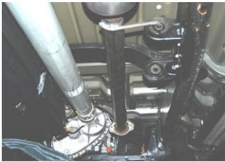
INSTALL HEADPIPE # A INTO STOCK PIPE. THE END OF THE PIPE SHOULD BE AT THE 12 O'CLOCK POSITION, ATTACH WITH BOLT KIT #I DO NOT TIGHTEN. INSERT WELDED HANGER INTO RUBBER GROMMET. REMOVE THE HANGER FROM THE FRAME & RELOCATE TO THE HOLES JUST TO THE LEFT OF THE OTHER HOLES YOU WILL NEED TO PRY THE INSERTS OUT & RE-INSTALL SFF PHOTO
