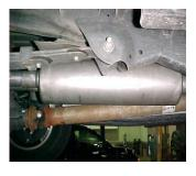
INSTALL MUFFLER # B ONTO HEADPIPE 1  $\frac{1}{2}$ " TO 2". USE CLAMP # F TO SECURE MUFFLER TO HEADPIPE. DO NOT TIGHTEN. USE A JACK STAND TO HOLD UP THE MUFFLER. OUTLETS SHOULD BE LEVEL.
