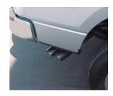
INSTALL YOUR BLACK CERAMIC COATED TIPS. PROCEED TO THE NEXT SHEET ON HOW TO INSTALL YOUR DEEGAN 38 BADGES. AFTER YOU HAVE CHECKED FOR CLEARANCES GO BACK AND TIGHTEN ALL NUTS, BOLTS AND CLAMPS.
