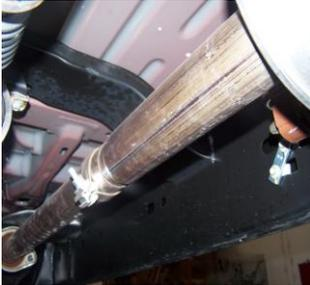
TO REMOVE YOUR STOCK EXHAUST, REMOVE IT FROM THE CLAMP LOCATED JUST IN FRONT OF THE MUFFLER REMOVE HANGERS FROM RUBBER GROMMETS BY PULLING EXHAUST TOWARDS THE REAR OF THE VEHICLE, USE WD-40 TO AID IN REMOVAL, LEAVE GROMMETS IN PLACE.
