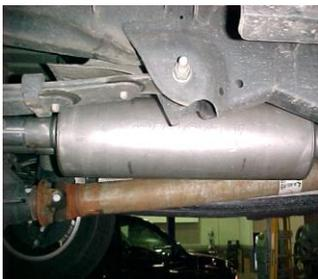
INSTALL MUFFLER # B ONTO HEADPIPE 1 1/2" TO 2". USE CLAMP # F TO SECURE MUFFLER TO HEADPIPE. DO NOT TIGHTEN. USE A JACK
