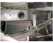
ON DRIVER SIDE: ATTACH REAR TAILPIPE HANGERS #I TO FRAME BY REMOVING THE 18MM HITCH BOLT. THEN RE INSTALL BOLT WITH HANGER (IF YOU DO NOT HAVE A FACTORYHITCH USE BOLT KIT #L TO ATTACH HANGER #I TO THE FRAME RAIL. REPEAT ON PASSENGER SIDE.
