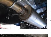
**3.INSERT REAR MUFFLER HANGER** INTO CORRESPONDING RUBBER
