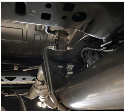
3. with Muffler in place install your over axle pipe. Keep everything loose until all is installed. Be sure to not bottom out the hanger into the factory grommet. It will create vibration.
