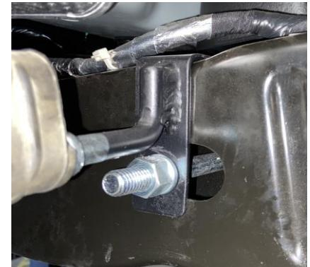
2. Install Headpipe Item # A onto the factory flange using factory bolts. Install muffler with louvers opening towards the rear of the vehicle. Facing them forward will reduce sound levels and quality of sound.
