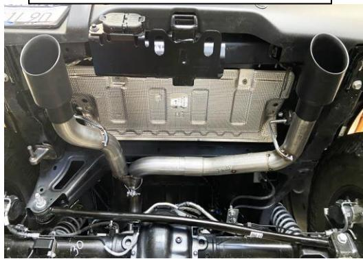
5. Install the y pipe and insert the hanger into the factory rubber grommet on the supplied Gibson hanger. Install the driver side pipe as well. Keep in mind the length the pipe is slid on will change the angle of the tip. Make adjustments until it fits correctly.
