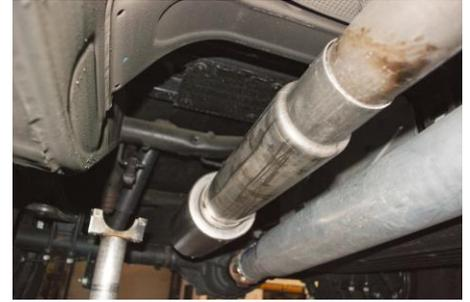
2. **Note: 2009 models** will not have the 2-bolt flange and will require the adapter Item# G. Measure 8.0" from the flange on head pipe item # A and cut. Attach the adapter to the new head pipe using clamp item # E. loosely tighten down and install
