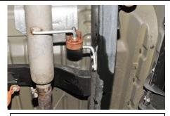
3. With the muffler assembly installed you may want to use a jack stand to support the muffler while installing the over axle pipe.
