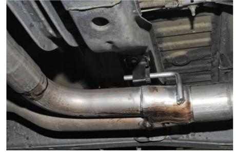
4. Install the Resonator Item #B onto the head pipe Item # A. The inlet of the resonator will have the louvers opening towards the front of the vehicle. Loosely tighten down.
