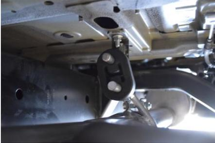
2. Install Head pipe Item # A onto the factory flange. Install hanger into rubber grommet and loosely tighten down the flange. 4wd use (K) to bolt in hangar mount.
