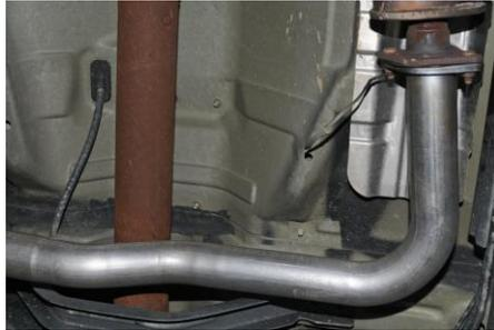
3. Install Head pipe Item # H onto the factory flange. Slide the head pipe into item # A before attaching the two bolts. Loosely tighten down.
