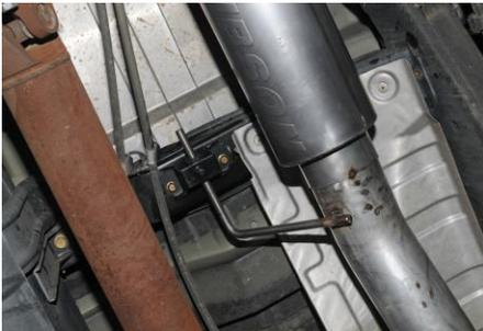
5. Install The muffler assembly Item # C Onto the resonator. Also slide the muffler hanger into the factory rubber grommet. Install the over axle pipe Item # D into the muffler outlet and install the hanger into the rubber grommets. Use clamp Item # F to secure. Do not tighten
